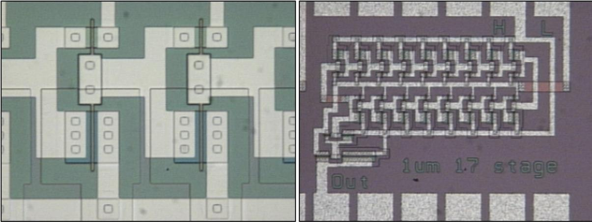
The SMFL has a 2um CMOS process with an effective L of 1.5um.
